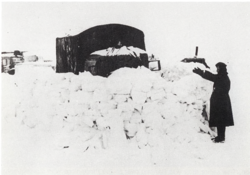
German lorry drivers build igloo walls around the engines of their lorries to protect them from the powerful icy winds which bring sub-zero temperatures.
