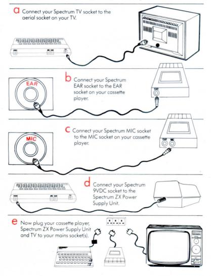
Switch on your TV and turn the sound down to its lowest setting. Find your computer channel. When SINCLAIR RESEARCH appears on the screen, you have found the right channel. If SINCLAIR RESEARCH does not appear on any channel, you will have to tune one of the channels. Refer to your TV manual for instructions on how to do this.
