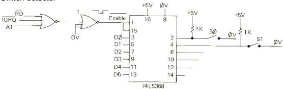
Switches S2 to S5 are similar to S0 and S1, each with a 1K resistor, and are connected to pins 6, 10, 12 and 14.
